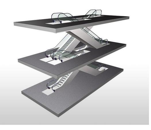
Continuous arrangement allows the fastest movement of passengers over two or more floor levels, so is particularly suitable for public service buildings, office buildings or large department stores
