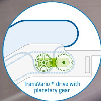
TransVario™ drive with planetary gear
